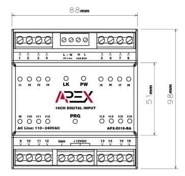
The APEX DIN-Rail isolated 16-channel digital input module is designed for seamless integration with APEX DIN-rail modules or MINI-IP via the CAN-BUS network. This robust module features LED indicators for each channel, providing clear and immediate status updates.
