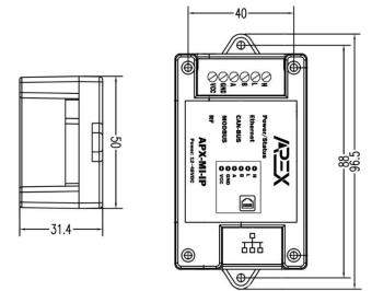
The APEX Wall Mounted MINI-IP Gateway is a compact and intelligent solution designed to seamlessly integrate Modbus and CAN-BUS devices into modern smart home systems. Ideal for connecting thermostats, industrial sensors, and other Modbus devices to home automation centers like Control4 and Fibaro, this versatile gateway also facilitates the connection of CAN-BUS APEX devices to Ethernet ports, enabling smooth communication with home centers.
